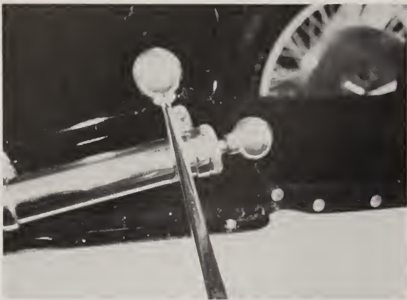
This hand pump—likely an oil pump—manually moved the lubricant to the top of the engine when the engine was hot and needed the oil most. The splash lubrication did little to keep the engine lubed and cooled. Ray Touriel
