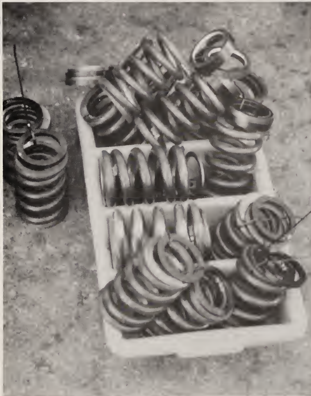
Springs are sorted and arranged according to tension. Teams are occasionally forced to change springs in the pits... not a chore the crew looks forward to. Notice the difference in thickness of the spring material.
