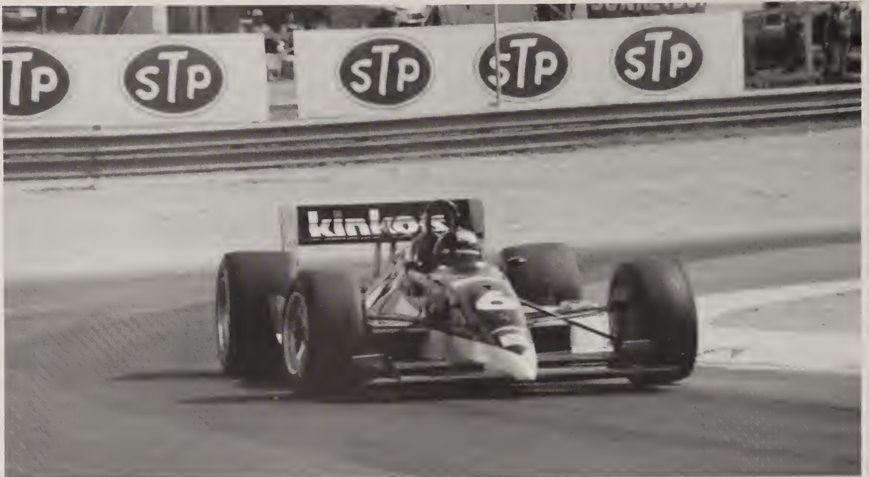
Didier Theys' Lola has its wheels slightly cambered, with the tops of the wheels a few degrees closer together than the bottoms. The car tends to be more responsive—but also more difficult to control
