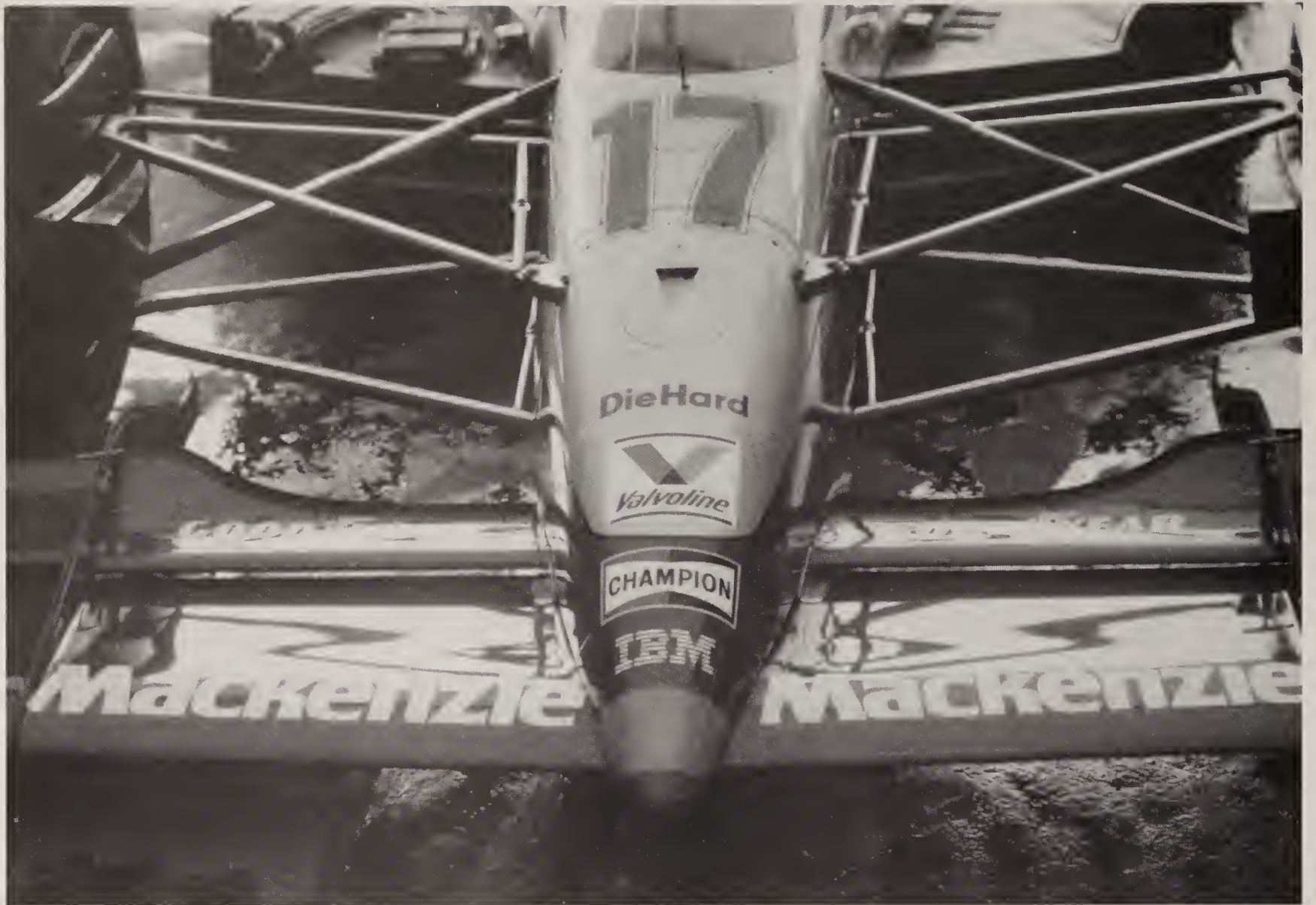
Strong but light, aero tubing helps reduce the car's drag, yet crew men can actually stand on it. It is relatively aerodynamic stuff as well.
