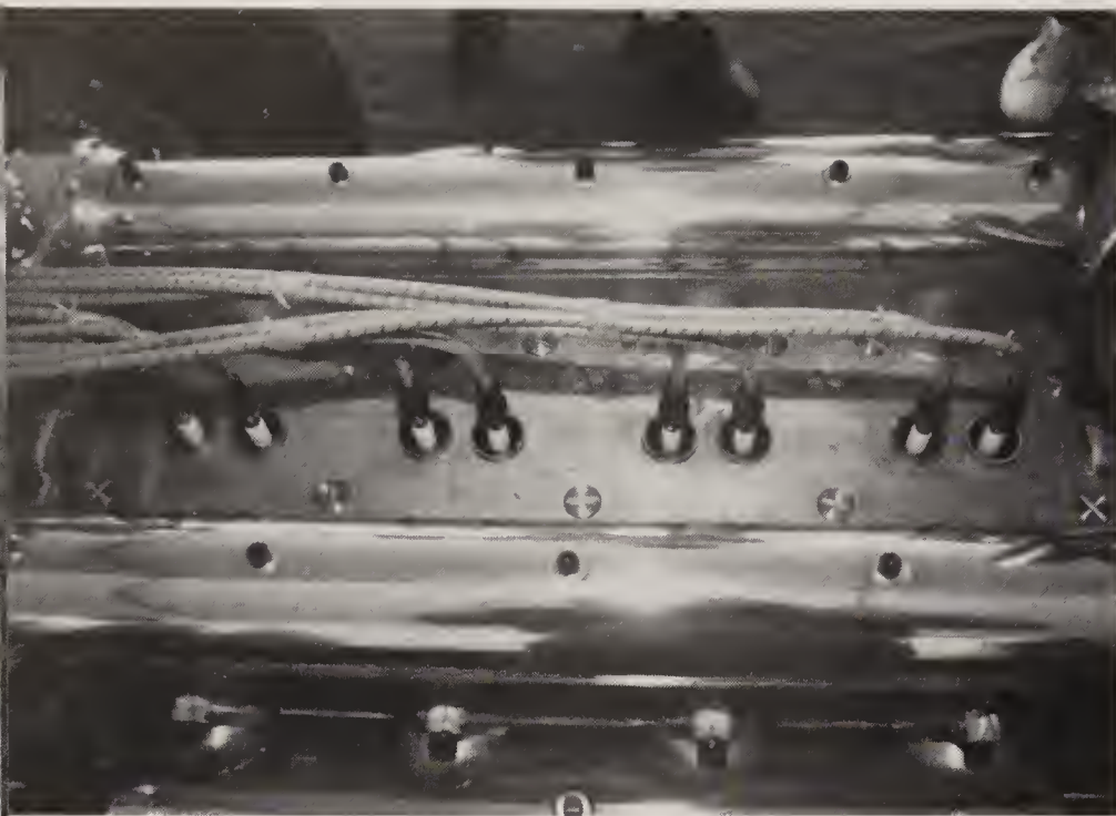
The Miller "91" engine, an in-line eight cylinder 90.2ci 285 horsepower supercharged powerplant. The 91 was supercharged and had a hemi-head design—very progressive for its time. The 91 is far simpler looking than its less powerful, larger counterparts, the 182 and the 121. The 91 won the 1926 Indy 500 with Frank Lockhart at the wheel. This one is non supercharged, with dual carbs, mounted on the right side of the engine. Deke Holgate, Pennzoil Public Relations
