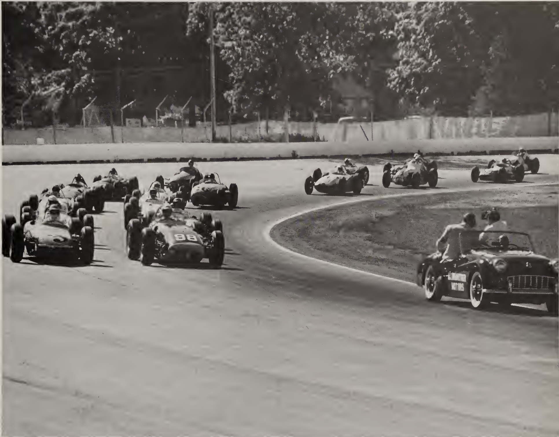
The start of a 1960 Indy Car race when the roadster dominated the field. Notice the offset driving position of the number three car on the outside front row. The offset cockpit defined
