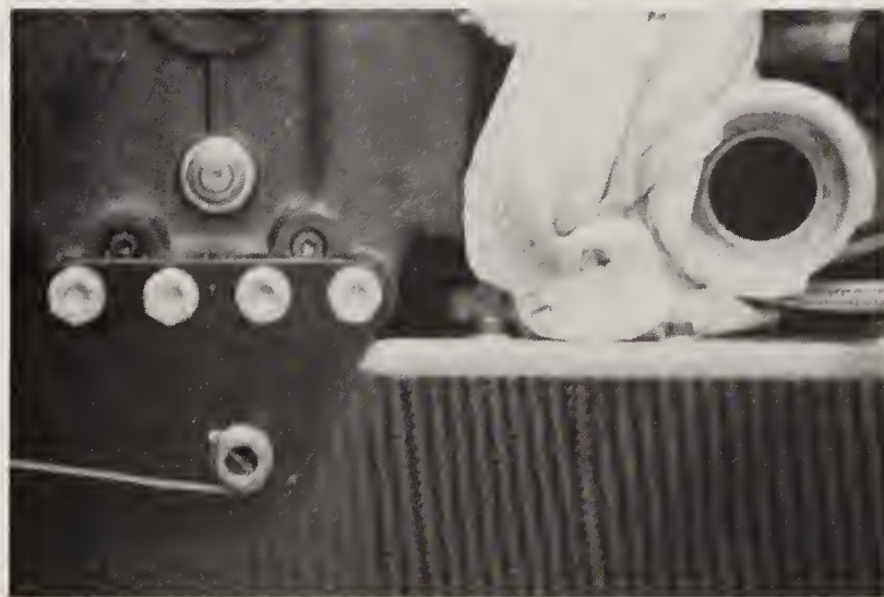
The engine is attached to the chassis by just a few bolts. The engine is actually a stressed member of the chassis, bearing the loads of the entire platform of the race car. The chassis is essentially the cockpit and all the mounting points of the suspension. Nevertheless, it is the chassis design that can truly make or break a season.
