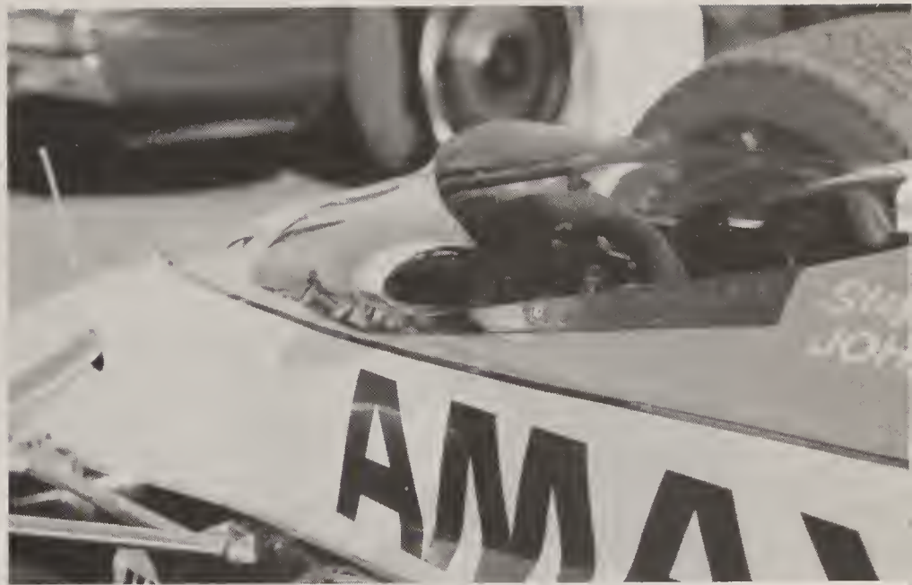
The bodywork is slimmed down for the lowest possible drag coefficient. Drivers tuck down into the "tub" to stay out of the wind and reduce drag; only the very tops of their helmets are prone to catching any wind. Modern helmets are designed to minimize drag and keep the buffeting of the driver's head to a minimum.
