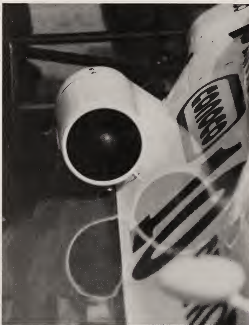
The Truesports car used a different setup for turbo intake in 1992. Turbo inlets on most cars are incorporated into the bodywork as slits or ducts. Here, the intake hangs out of the bodywork. The designers must hope that the benefits of the turbo more than offset the aerodynamic price paid for a component that sticks out into the air like this.
