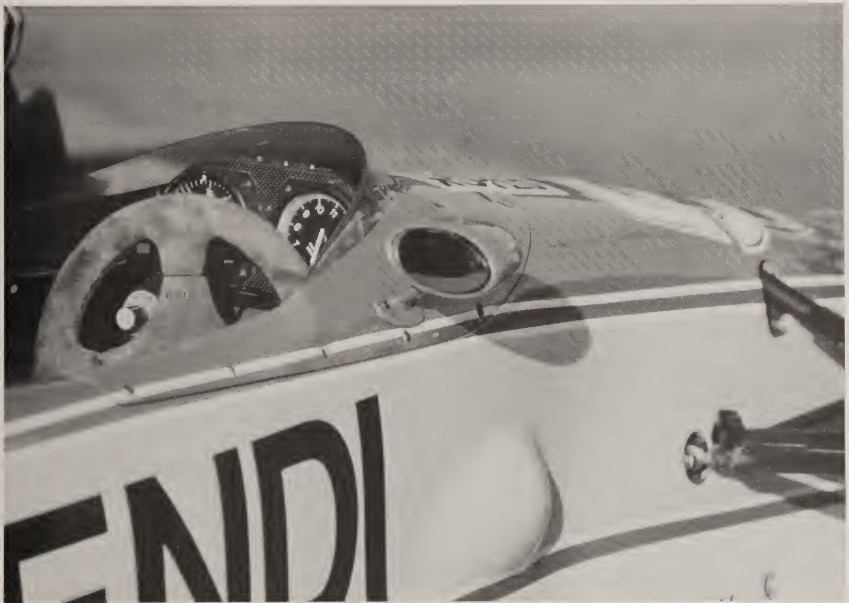
Despite the tight driver compartment, the driver still needs room to shift. Notice the bump in the bodywork to accommodate the driver's hand. Anything that sticks out into the wind
