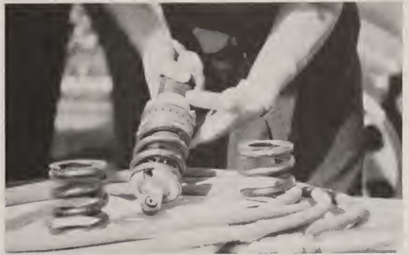
Springs are fitted over the shocks. The threads on the top of the damper can be adjusted effectively lengthening or shortening the pushrod to lower or raise the ride height of the car. One-sixth of a turn of that nut can make a big difference in ride height.
