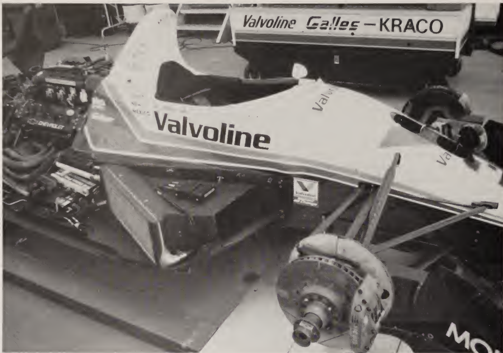
Under the sidepod covering—wherever it fits, the electrical system is mounted as if it is an afterthought, yet it does one of the most significant jobs of any component on the car.
