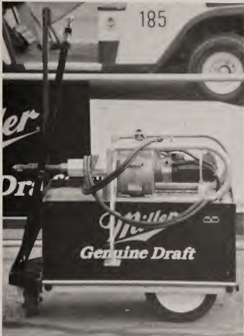
The starter is always available. Should the driver stall the car in the pits during his stop, the crew will quickly move toward an external starter such as this one to re-fire the motor.
