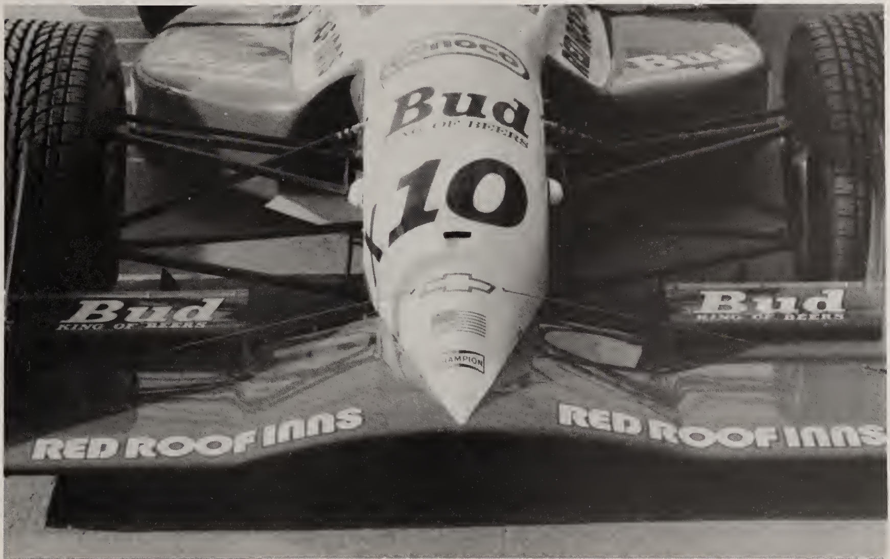
Here is the 1992 Truesports chassis design. The front wings are equipped with different flaps that can be added or taken away and which have different angles so teams can raise low-
