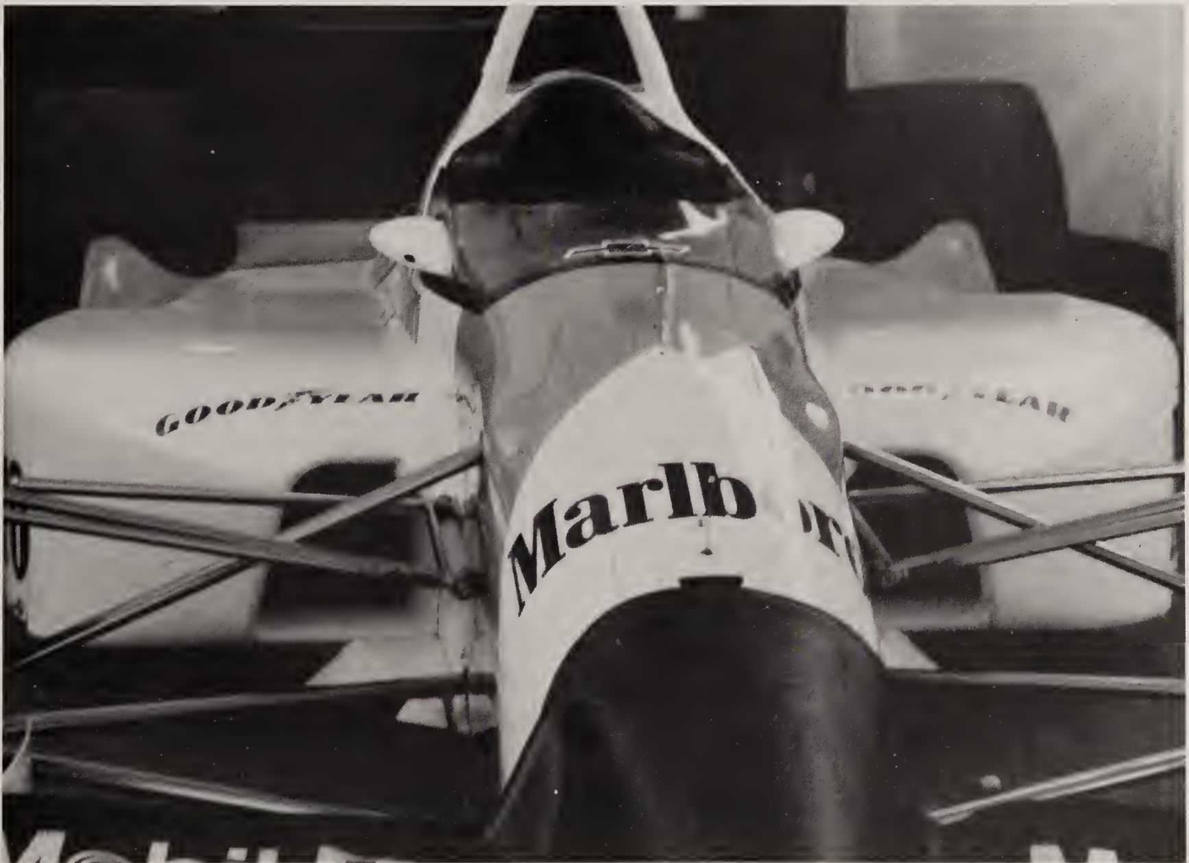
One of the Penske's configurations. Note the small radiator inlets. The danger with such a design is that if the weather gets too hot, the car tends to overheat. Compare these small inlets to those of other cars seen throughout this book.
