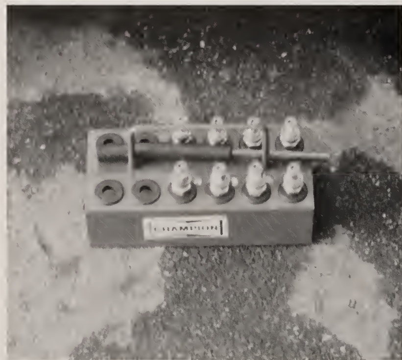
Spark plugs used in Indy Cars are similar to any street car plugs. "Reading" the plugs is not really a viable way to determine what is happening in the engine anymore—at least not with current technology. Instead, there's a wealth of data provided by the cars' electrical systems, which monitor practically every aspect of performance.
