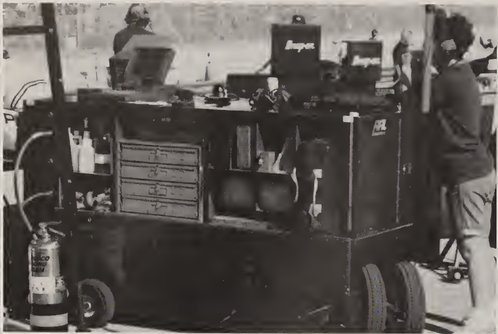
One of the many ways to package spares. This mini-trailer contains mostly electronic equipment which will be used as a link to the car while it's on the track. After a practice run, systems numbers might be crunched and scrutinized on these screens before adjustments are made.
