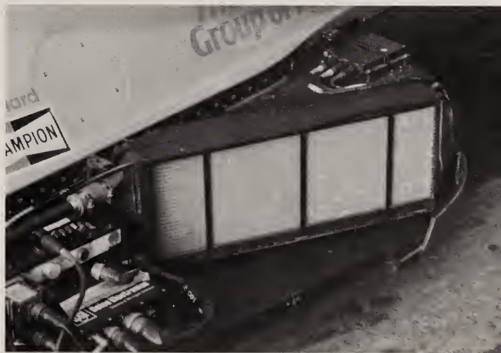
The cooling system features a pair of radiators. This one is exposed here, but they sit inside the side pod bodywork when the car is on the track. Cool liquid is pumped through the bottom of the engine and flows upward.
