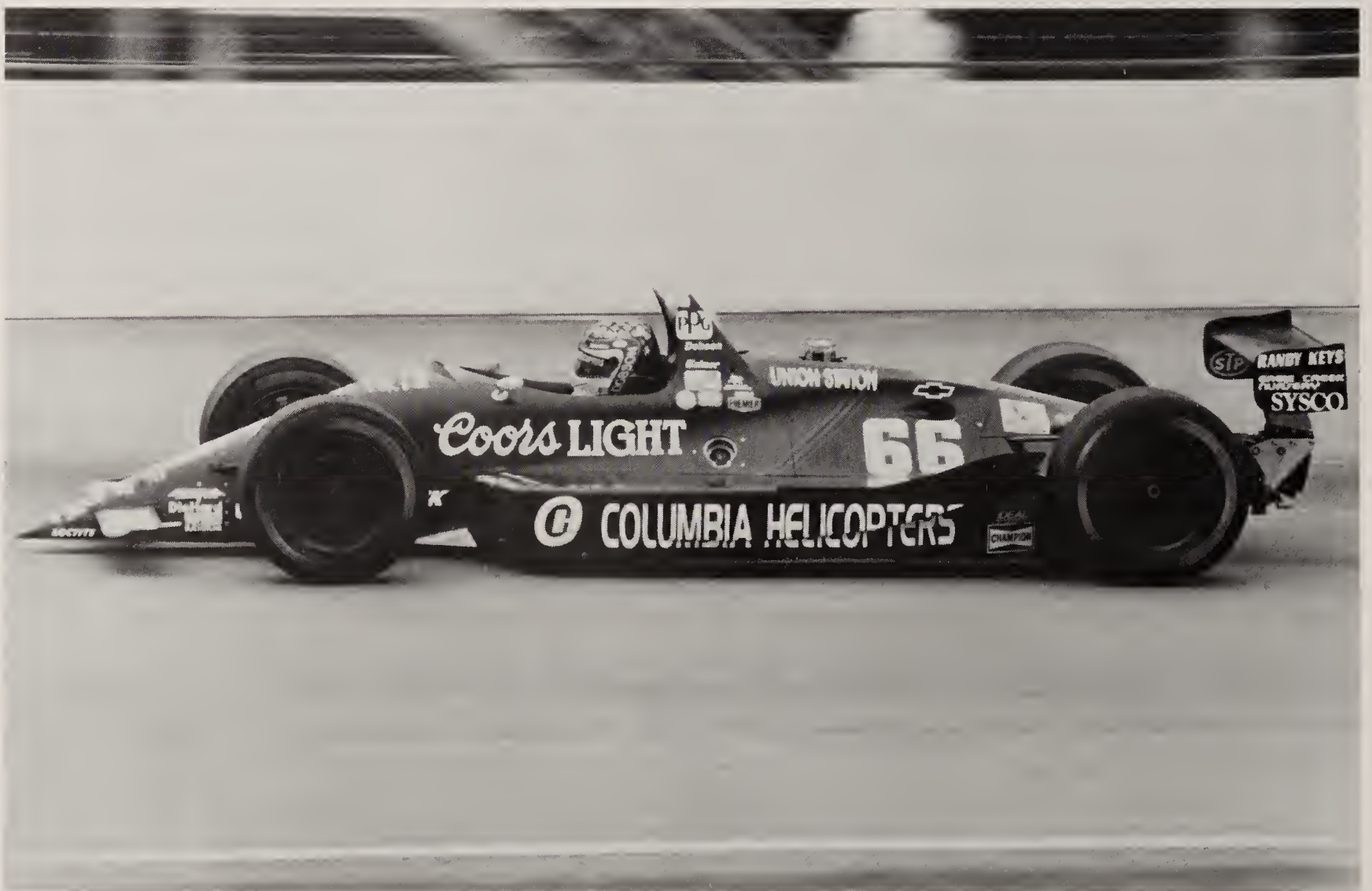
Dominic Dobson at speed at Indy. Compare his car's speedway set-up to the road course set-up of Mario Andretti's car in the previous photo. By comparison, Dobson's car has extremely small wings, front and rear. The back side of his helmet is
