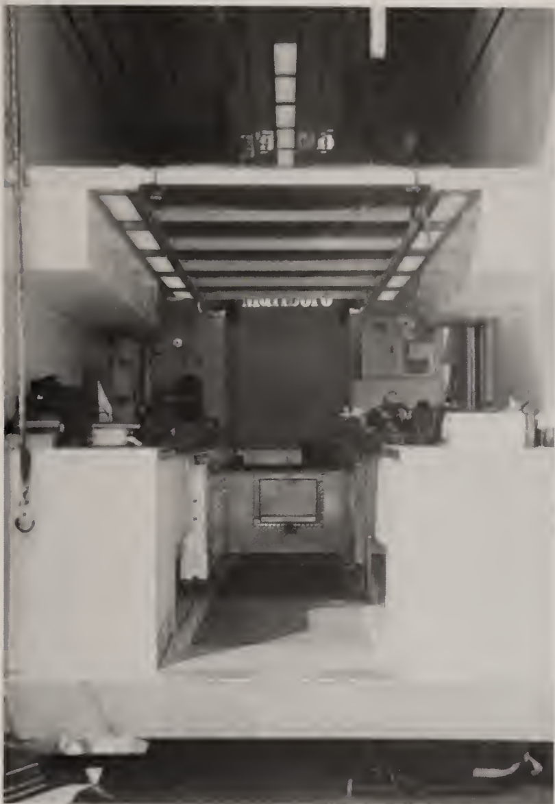
The transporter holds just about every possible spare part the crew could need. The split level holds two cars, spare engines, and serves as a self-contained workshop.
