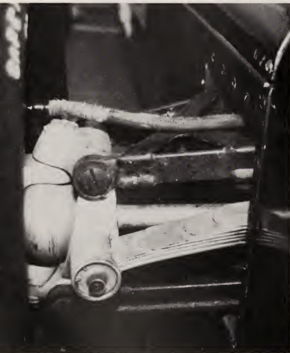
Hydraulic brakes on Louie Meyer's 1936 Miller-Stevens Indy 500 winner. The units were prone to overheating and both bad fade and malfunction. Thankfully, they were not used often in an oval track race. Ray Touriel
