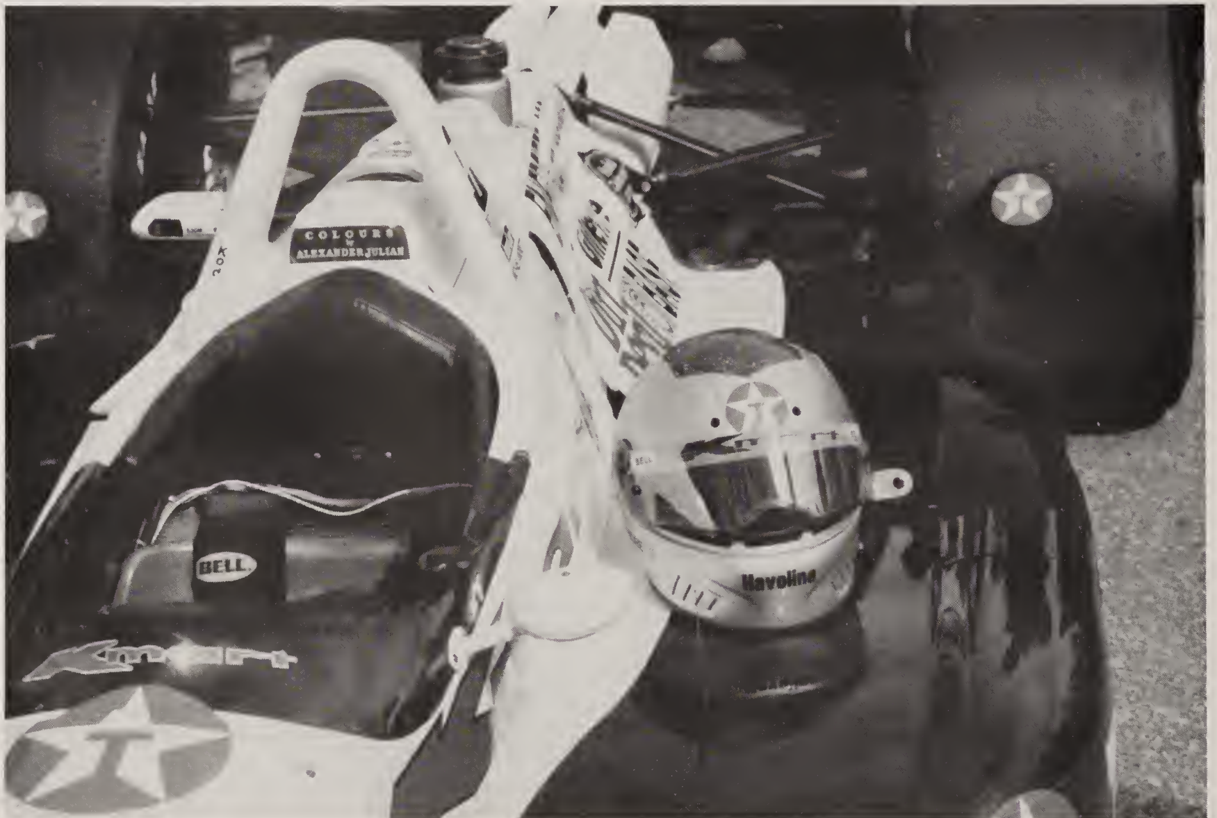
The car awaits Mario. The small white box sticking out to the left of the roll bar is the in-car camera; the small dark space on the box is the lens opening. His helmet is designed to be as aerodynamically efficient as possible. The small tab sticking
