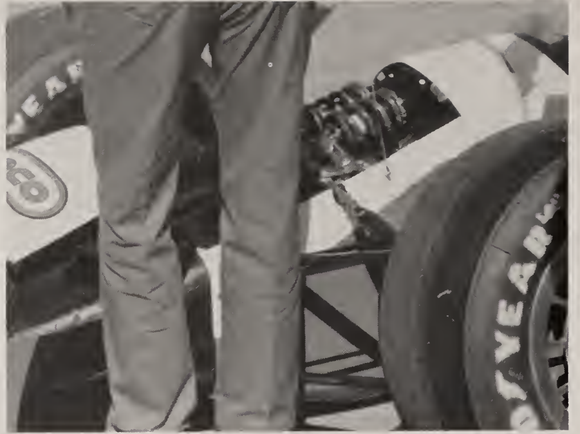
Note the rocker linkage in this photo. As the wheel moves up vertically, the rocker pushes the lower arm in, which activates the spring and damper. The anti-roll bar is attached via a link to the other damper and control arm.
