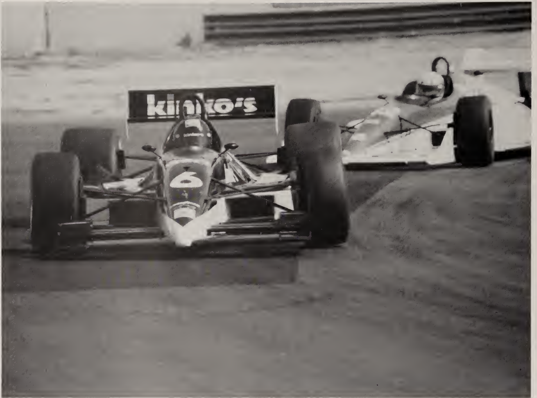
Tire wear is a function of the track, and part of a driver's savvy is his ability to save the tires. In this photo, the wear on the left front tire on Didier Theys' car is obvious.
