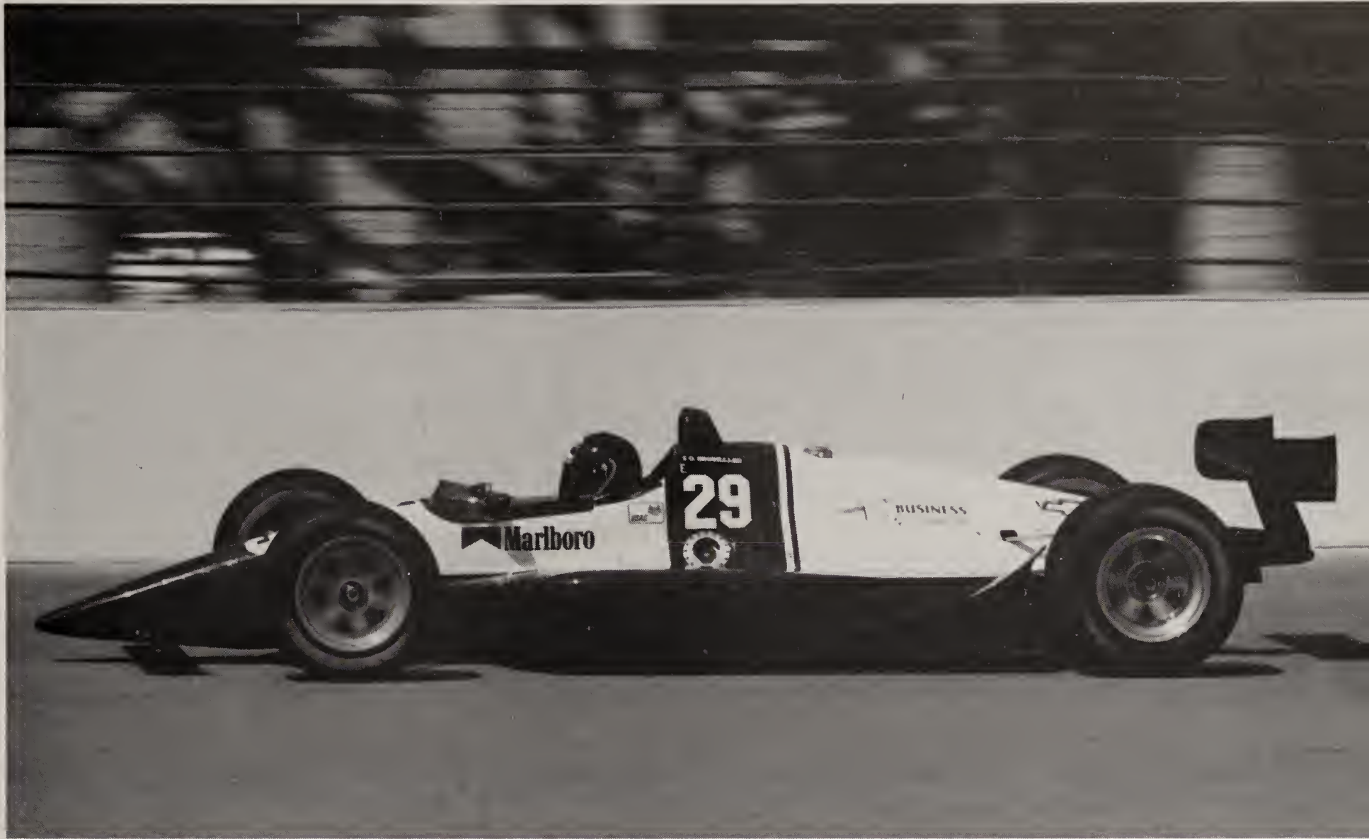
The superspeedway set-up. Notice the limited down force on the speedway kit; actually, there is very little down force. The
