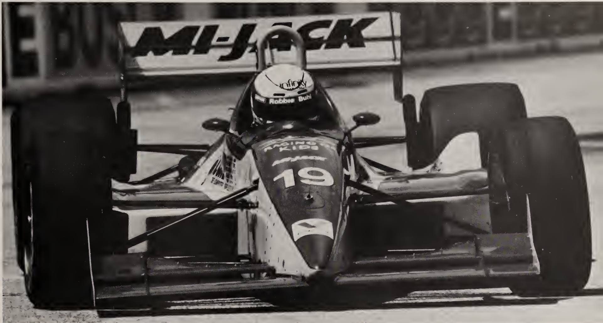
Notice how the wheels are toed in—pigeon toed—on Robbie Buhl's car. On a street car you expect to see the wheels pointed dead ahead while the steering wheel is set straight ahead.
