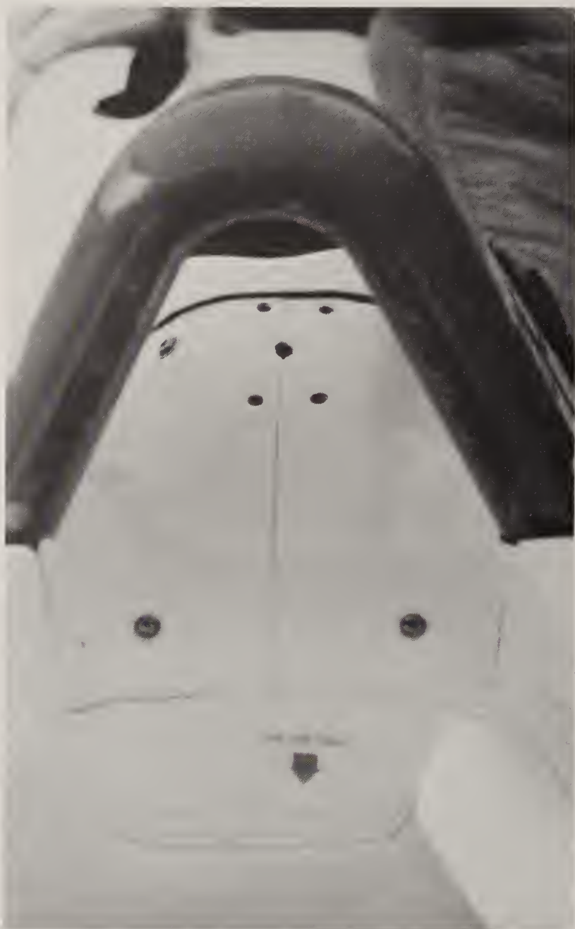
The roll bar, uncovered. Ernest Hemingway once said race car driving and bull fighting were the only two true sports. The similarities between the two speak for themselves—but bull-fighters no longer have tech inspectors and safety commissions. Today's roll bars double as loops for tow trucks to hook on and lift disabled cars off the track after breakdowns or mishaps. There's nothing less pleasing for a driver than to see his car on the end of the hook, a signal that, for him, the race is over.
